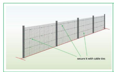
Step 10: Attach Mesh to Tensioning Wire
