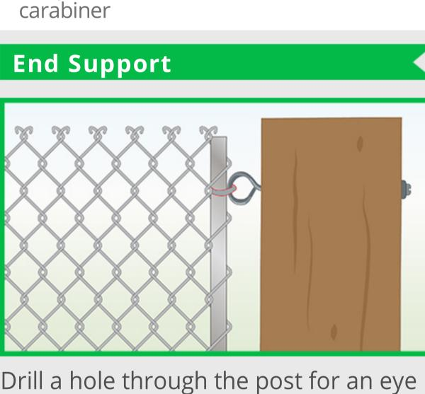
bolt. Secure it with a washer and nut,
