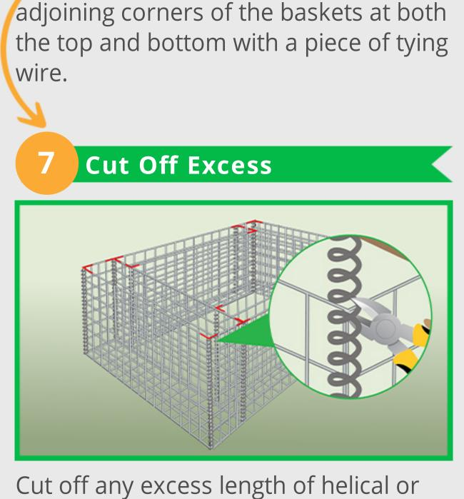
tying wire as needed using wire cutters
