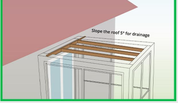
Affix a batten to the back of the structure, then add several more perpendicularly on top to create a proper slope for water drainage.
