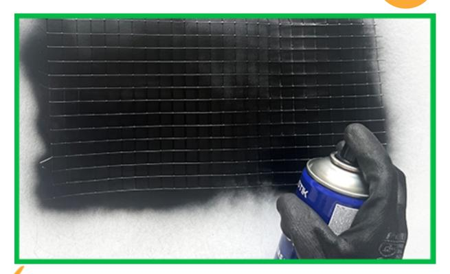
Flip the mesh and apply another even layer of spray paint.
