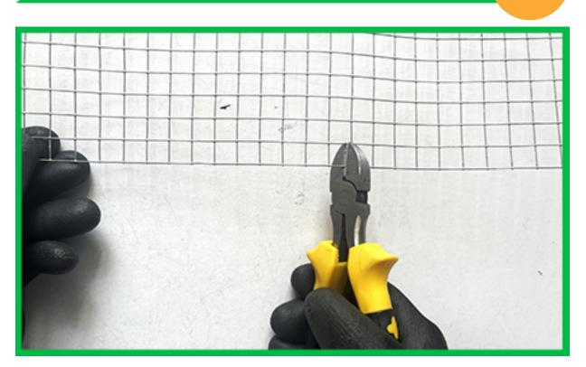
Use wire cutters to cut the mesh to your desired dimensions.
