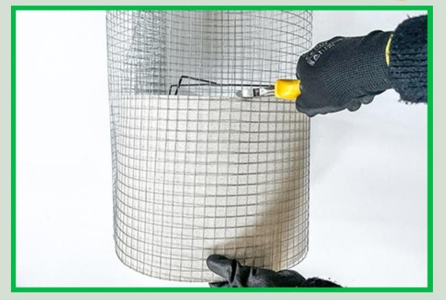
Once secured, you will see how much of the mesh needs to be cut. Cut the mesh to size using wire cutters.
