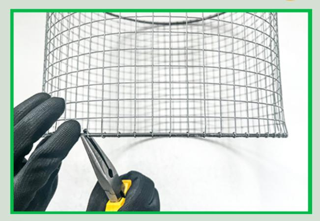
Use pliers to wrap the ends of the mesh tightly around the hoops. Repeat this on both the top and bottom of the lamp shade.
