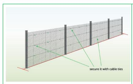
Step 10: Attach Mesh to Tensioning Wire
