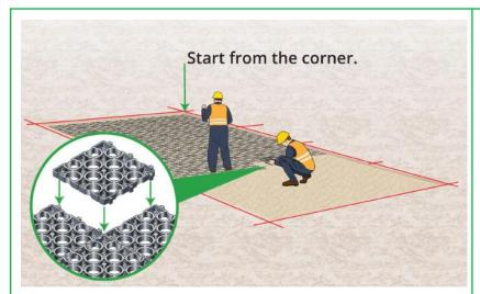
**Step 7:** Starting from a corner, place the plastic driveway grids on top of the sand interlocking them together.
