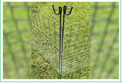
**Step 8:** To easily open and close the door, you should have a fence pin in both panel connectors, one pushed into the ground at all times and the other one pulled out just enough to allow for movement.
