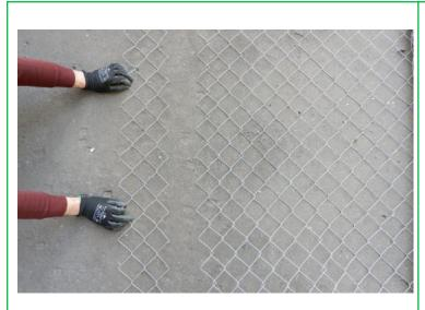
**METHOD A - Step 4:** After you're done removing the offcuts, pull the separated section away from the rest of the roll.
