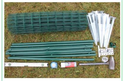
**Step 1:** Gather and lay out the PVC coated wire mesh fence kit and the tools you will need.
