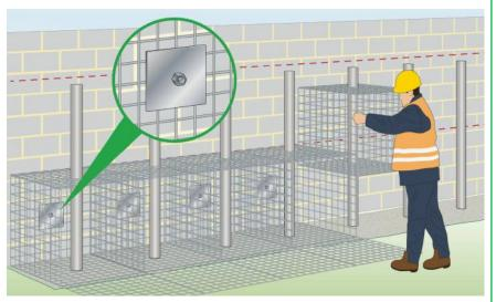
**Step 7:** Place the cages on top of the beams. If the diameter of your support beams is larger than the 75mm x 75mm holes in the mesh, then you can use bolt cutters to create a bigger hole.
