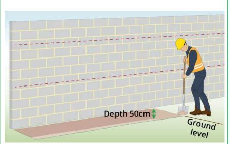
**Step 3:** Dig a trench directly under the location of the cladding. This is where your support beams will be located.
