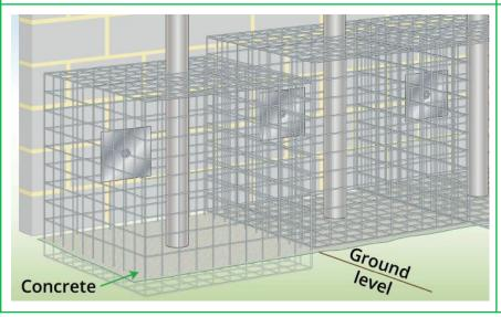
**Optional Step 1:** For added stability, you can install the first row into the ground/concrete.
