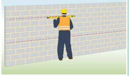
**Step 2:** Mark the exact location where you plan to install using a spirit level or laser level to ensure it is straight.
