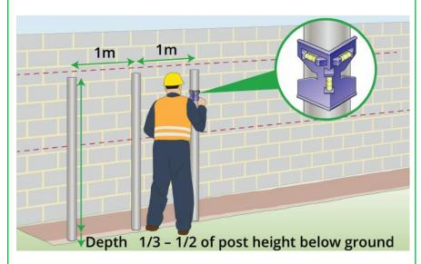
**Step 4:** Using a spirit level, place the support beams at 1m intervals directly under the location where the baskets will be installed.
