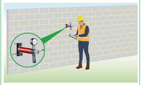
**Step 1:** Assess the structure where you are intending to attach the cladding, to ensure it can hold the weight of the gabions.
