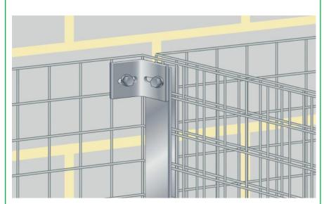
**Optional Step 2:** For added stability, you can also install an angle section and clamp bar.
