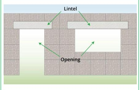
**Optional Step 3:** Where an opening is required for doors or windows a suitable lintel will be required.
