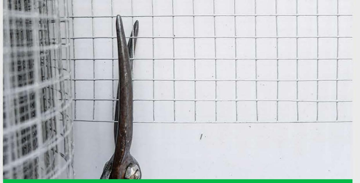
Knowing the length you need to use, cut the mesh down with tin snips, wire cutters or even scissors if it's thin enough. Pull away the roll from the cut down section.
