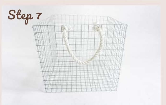
Take a length of rope which fits in the hole size of the mesh. Push the two ends of rope through the hole sizes of the drawer and knot both ends so they don't come out when you pull on the handle.
