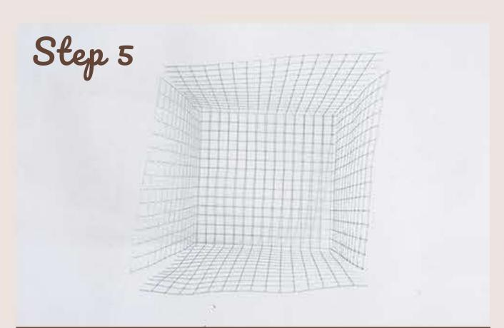
After you cut the wire mesh to size, use a hard object that fits inside the 4 sides of the baskets to fold up the sides. Push down the object and fold up the sides alongside the base of the drawer until they meet vertically.
