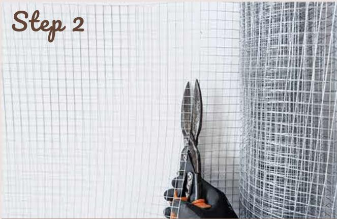
Take a roll of mesh and roll out enough length to cover the drawer's dimensions stretched out. Have a partner help you to hold the roll in place. Cut the required mesh length carefully with tin snips.
