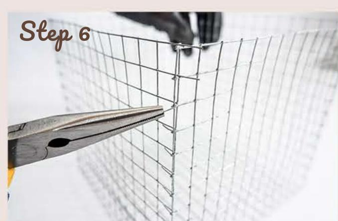
Take a needle nose plier and start wrapping excess wire around the edges of the drawer. Fold in all the wires on all corners, making sure that you secure them properly and that they don't poke out.
