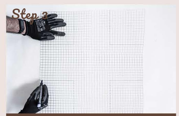
Draw the stretched out drawer on the mesh knowing the dimensions. Make sure that you mark the same height and length for all sides. It is advised to mark along the wires so it is more visible.
