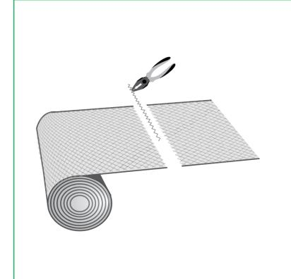
**Step 3:** Chain link can be cut to size but it's easier to shorten its length by detaching two sections.
