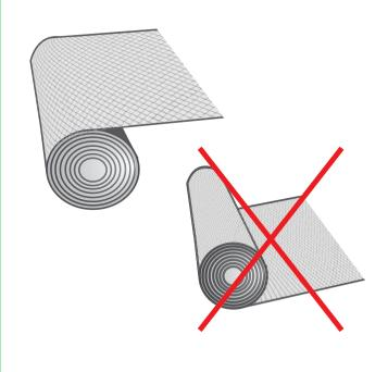
**Step 2:** Place the roll on the ground with the loose end upwards, facing in your direction.
