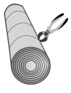
**Step 1:** Cut the tying wires that are used to fasten the roll and keep it from unraveling.
