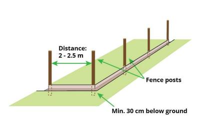
**Step 2:** Place your fence posts at even distances of about 2-2.5 meters. Make sure to have one at each corner of the area.
