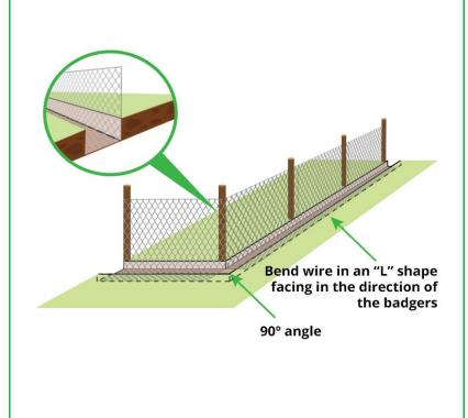
**Step 6:** Continue attaching the mesh to the rest of the posts on the other sides of the area, while also bending the bottom to create the 'L' shape facing outwards.
