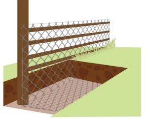
Attach any type of wire or plastic mesh to the top of the fence at a 45 degree angle to make extra sure the animals can't get through.
