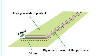
**Step 1:** Dig a trench around the perimeter of the area to a 30-60cm width and a 30cm depth.
