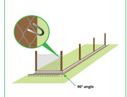
**Step 4:** Cut a length of mesh enough to cover the distance between the first two corner posts, and bend the bottom 30-60 centimeters at a 90-degree angle, creating a flap facing outwards.
