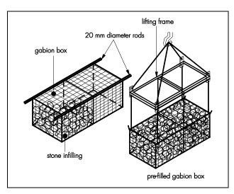
Figure 9 Safe lifting of prefilled gabions from the base
