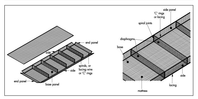
11.14 Ends, side panels and diaphragms are lifted into position and the ends and diaphragms are secured to the side panels using the method indicated in section 11.3.
