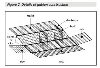
11.2 Front and rear sides, ends and diaphragms are lifted into position to form a box shape.
