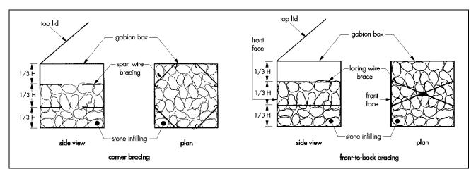
11.6 The gabion boxes are filled with suitable stone such that the mesh lid bears down on the stone. If large voids are present, these should be infilled with small stones.
