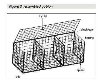
11.4 A number of empty gabion boxes may be placed in position on a flat surface and secured together with spirals, 'C' clips or lacing wire, starting from the top corner in a continuous operation using alternate single and double twists at a maximum spacing of 100 mm (see Figure 4).
