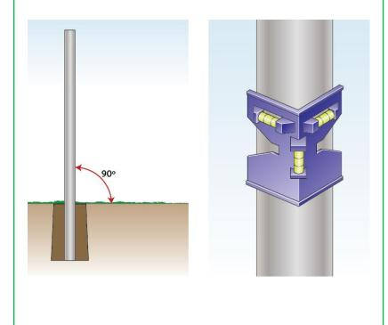
IMPORTANT: Use a level to make sure the post is straight then secure it in place. This is important otherwise your fence will not be straight.
