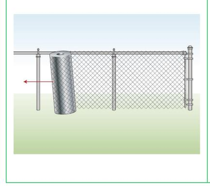
Pull the mesh roll tight along the length of the fence removing any slack. At this point you only need to remove slack, you are not permanently tightening the fence yet.
