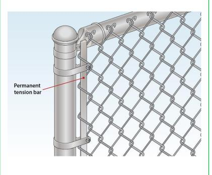
Weave the permanent tension bar through the mesh and tension bands attached to the remaining end pole. Then tighten the tension band nuts and bolts. Then remove the temporary tension band.
