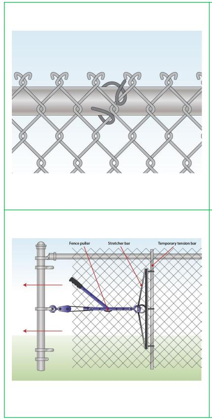
Add a few wire fence ties to attach the mesh to the top rail.
