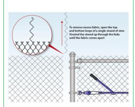
As you tighten the mesh there is likely to be excess mesh that you will want to remove. Unravel a strand of wire from the mesh to remove the excess.
