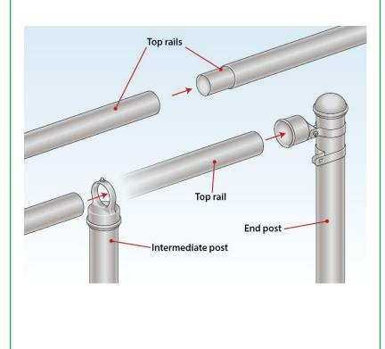
**Step 5:** Push the top rails through the loops in the caps. The poles will attach to each other by pushing opposite ends together. If the poles are too long cut them with a hacksaw. Once the poles are in place, fasten all nuts and bolts.
