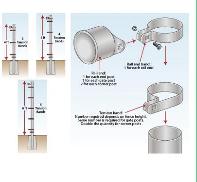
**Step 4:** Add tension bands to all posts with the flat side pointing to the outside of the fence. If you have corner posts you will need 2 x tension bands pointing to either side. You need to add one less tension band than the height of the fence, in feet. For example:
