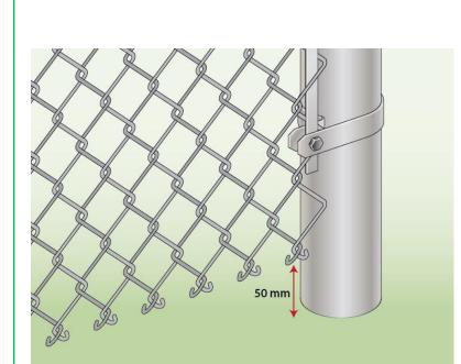
Attach the tension bar to the bottom tension band of the end pole. The mesh should also be 2 inches off the ground. If not adjust the height of your tension bands then tighten the bolts.
