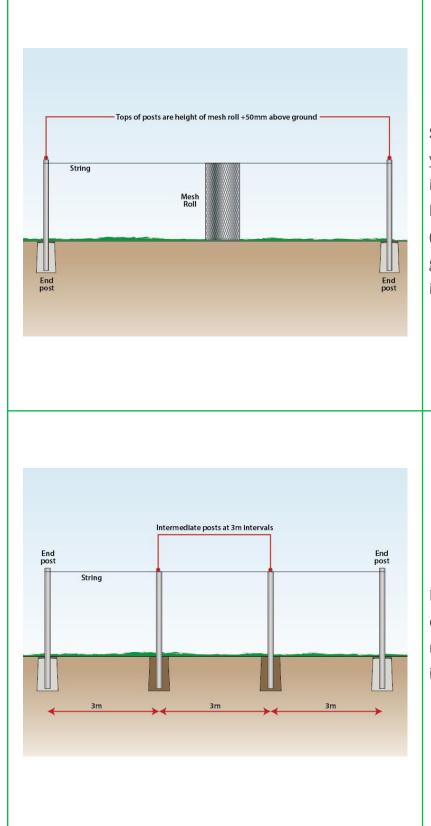
**Step 3:** Tie a string tight between your posts. The height of the intermediate posts should be the height of the chain link mesh + 50mm (2 inches) so that you have a small gap at the bottom of the fence once it has been installed.
