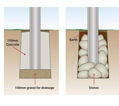
CONCRETE OPTION: For best results fill the holes with 4 inches of gravel and pat it down so that it is compact then add 6 inches of concrete on top. Then put the posts into the wet concrete and allow at least 1 day to allow concrete to set.
