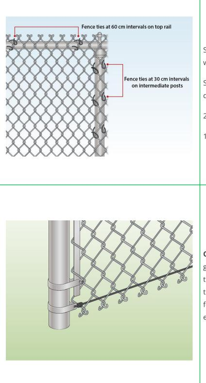
Secure the mesh to the rail and poles with fence ties
