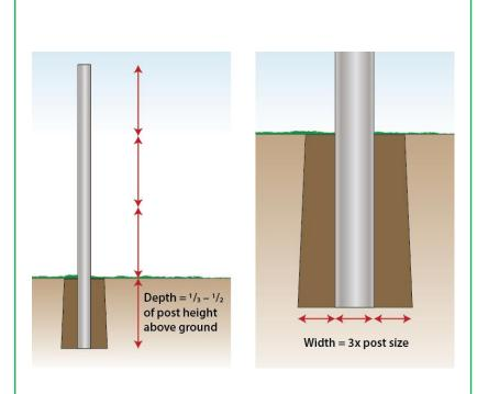
Dig a hole in each of the middle post locations. The holes should be three times wider than the post diameter. The depth of the hole should be 1/3 the length of the post.
