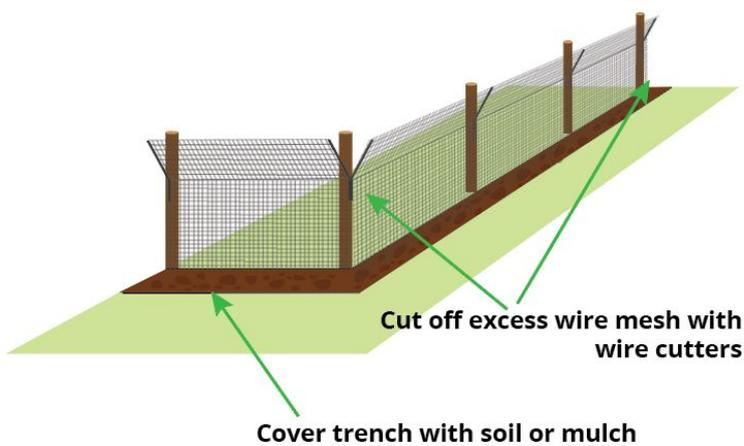
**Step 9:** Use wire cutters to remove any excess mesh. Check for any gaps in the fencing to make sure you get the best fox proofing results.
