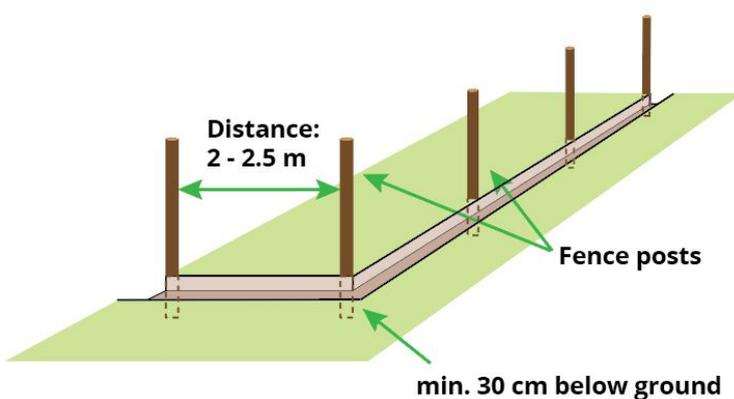
**Step 2:** Place your fence posts to an even distance of about 2-2.5 meters for effective fox-proofing. Make sure you have one at each corner of the area.
