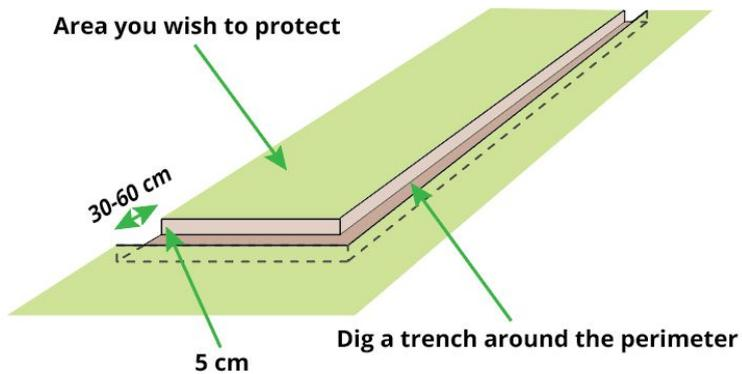
**Step 1:** Dig a trench around the perimeter to a 5cm depth and a 30-60cm width.
