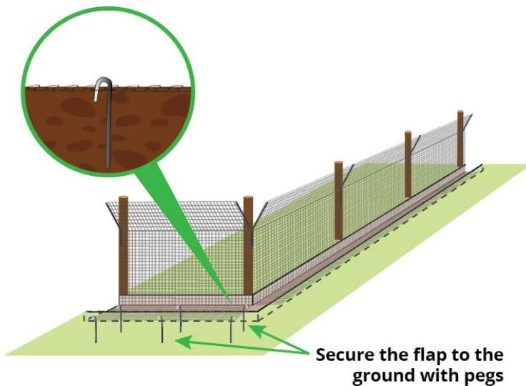
**Step 8:** Use pegs to secure the flap to the soil. Staple them right at the 90 degree angle and at the outside edge of the flap at about every 60 centimeters.
