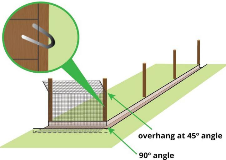
**Step 4:** Take a piece of wire mesh long enough to cover the distance between the first two corner posts. Bend 30-60 cm at the bottom of the mesh in an 'L' shape pointing outward, in the direction of the foxes. Bend the top 50 cm of the mesh to a 45 degree angle, creating an outward facing overhang.
