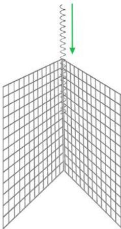
**Step 2:** Connect the panels by twisting the connectors down the joints.
