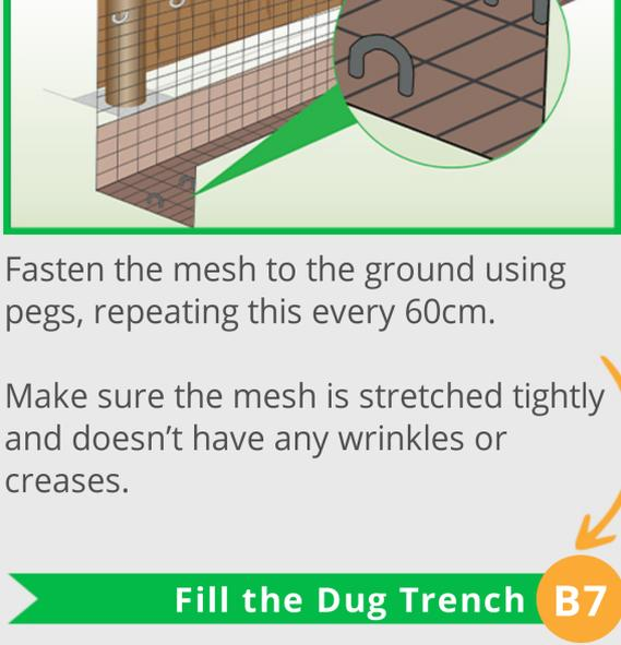
Measure the length and height of the installation area using a tape measure, taking into account the buried mesh in the 50cm depth and 30cm width trench.
