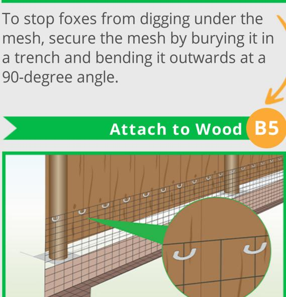
Take the soil you excavated earlier and use it to cover the trench, making sure to keep the mesh inside.
