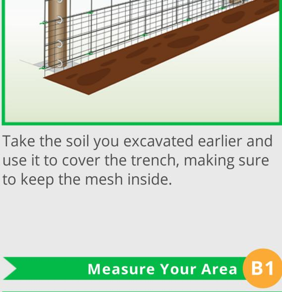
To stop foxes from burrowing under the mesh, make sure to bury the mesh deep into the ground and bend it outwards at a 90-degree angle.
